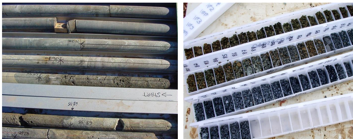
Figure 1. Drill-core (left) and reverse-circulation drill-chip samples (right) prior to preparation for analysis. Photo credit: MinAnalytical Laboratory Services Ltd.
