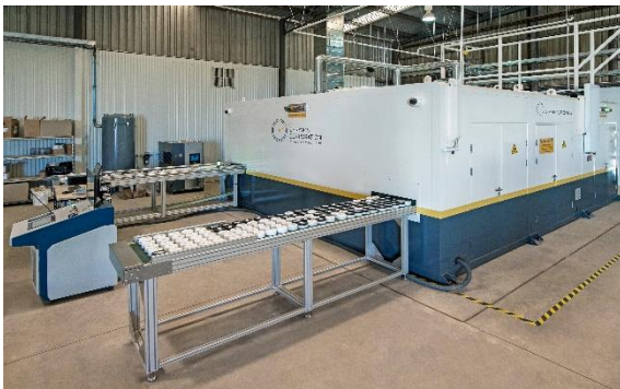
Figure 3. Photographs illustrating design of the commercial PhotonAssay Max system PA1408X. (Left) Overview of complete system, showing input and output sample conveyors, control console and cabins housing X-ray source, detector system and automation. (Right) Interior of automation cabin, showing reference discs and reference disc robot.
