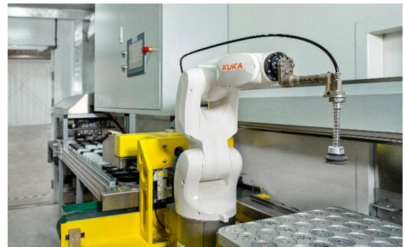
Figure 3. Photographs illustrating design of the commercial PhotonAssay Max system PA1408X. (Left) Overview of complete system, showing input and output sample conveyors, control console and cabins housing X-ray source, detector system and automation. (Right) Interior of automation cabin, showing reference discs and reference disc robot.
